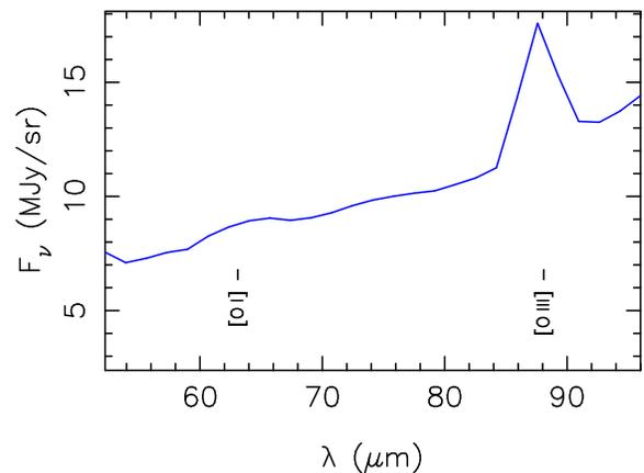
Figure 4: Actual spectrum of 30 Dor taken with MIPS/SED during in-orbit checkout. The [OIII] line is easily detected; the [OI] line is weak but can be observed in some positions.
